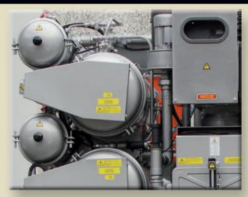
Multiple, independently functioning high-micron self-cleaning spin disc EcoFilters® and large-capacity carbon cartridge filters are available on all Union K Series Systems to assure optimum filtration of both large and small particles for maximum solvent purity. Computer controls automatically pair filter operation for whites, darks or colors according to specific programs.
